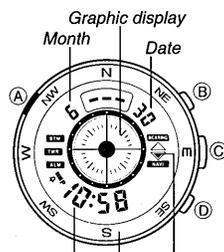
The Navigation Mode lets you store up to five sets of measurement data in memory. Each set of data includes the direction, along with the date and time of the measurement. You can later recall the memory data to trace your progress on a map.
