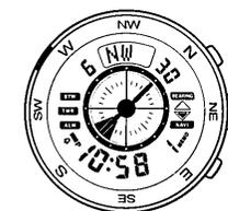
5. Next, you can adjust the rotary direction bezel so that the "N" mark is aligned with the magnetic north arrow. This correctly aligns all of the markings on the bezel.
