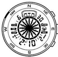
This indicator appears on the display whenever the Digital Compass has a problem obtaining a correct reading. This condition could indicate that the watch is within a very high magnetic field, and so you should try moving to another location. Also, see "Digital Compass Precautions" for further information on conditions that cause errors.
