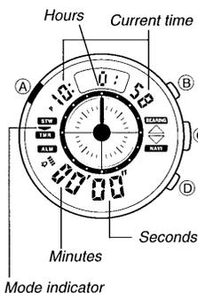
The countdown timer can be set within a range of 1 minute to 24 hours. When the countdown reaches zero, an alarm sounds for 10 seconds or until you press any button.
