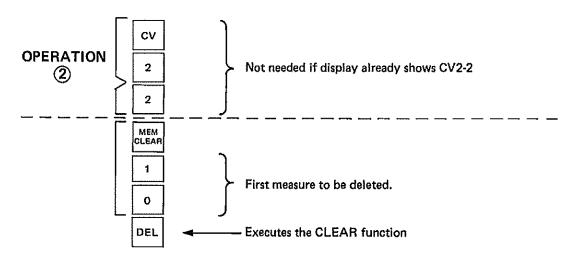
After pressing [ ] , the ADDRESS display will show the last step in M9; in other words, the display will show the last data now contained in CV2-2.
