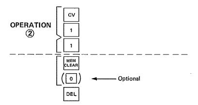
The above will activate the ERROR function indicating that the memory has been cleared of all data and the channel assignment cancelled.
