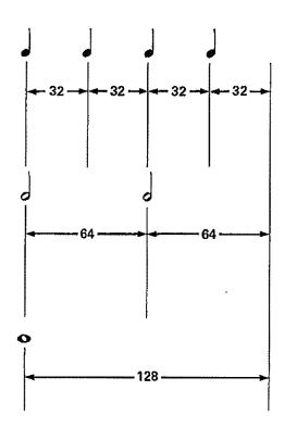
The actual length of time required for each increment will depend on the programmed tempo (see Section 14). In the above example, since a whole note equals 128, the smallest time increment we could program (a "1") would be equal to a 1/128 note. Also, the longest time value we could program into one step would be equal to two whole notes (128 + 128 = 256). For longer duration (such as tied notes) more than one step would have to be used as explained later in this section.
