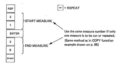
CYCLE switch off: Program will run once from M31-1 to the last step in M35. CYCLE switch on: The portion of the program from M31-1 to the last step in M35 will repeat endlessly (until see is pushed or CYCLE is turned off).
