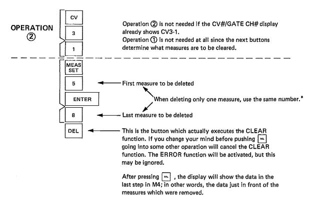
As the button implies, the data after M8 is brought forward to close up the hole left in the program by the CLEAR function.
