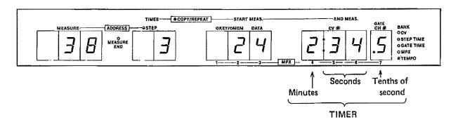
The timer is activated whenever the button is pushed and deactivated whenever the program ends or the button is pushed. This means that not only can the program be timed from the beginning to the end, but it can also be timed from any point to any other point using the RUN functions shown on page 72.
