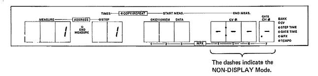
After the NON-DISPLAY mode, pressing will start the process over again from the beginning. Also, pushing some other button will interrupt the mode so that pressing again will start the whole process over again, rather than continuing with the next memory in line.
