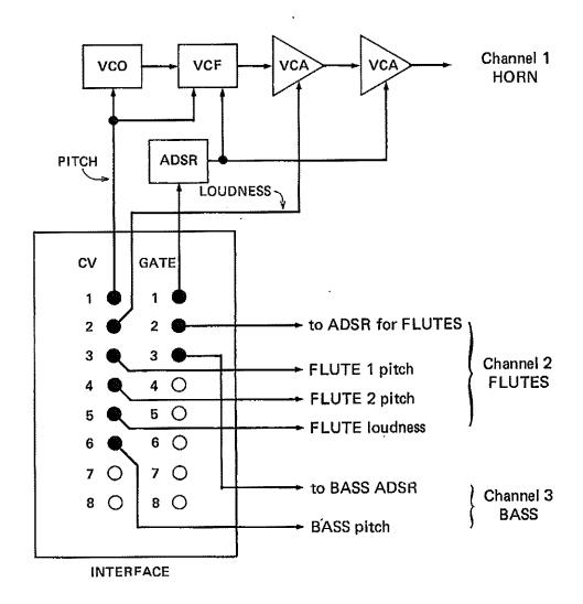
Each channel must contain one "S" (STEP TIME for note time valves) column as shown. In this example, the synthesizer is to produce four voices divided into three channels. Channel 2 contains two flutes of different pitches but controlled by the same gate pulse train. Note that two of the CV outputs are to be connected to VCA's for control of loudness. Control of the loudness of Channel 3 (in this example) is either not necessary, or it is to be controlled by one of the other CV outputs.
