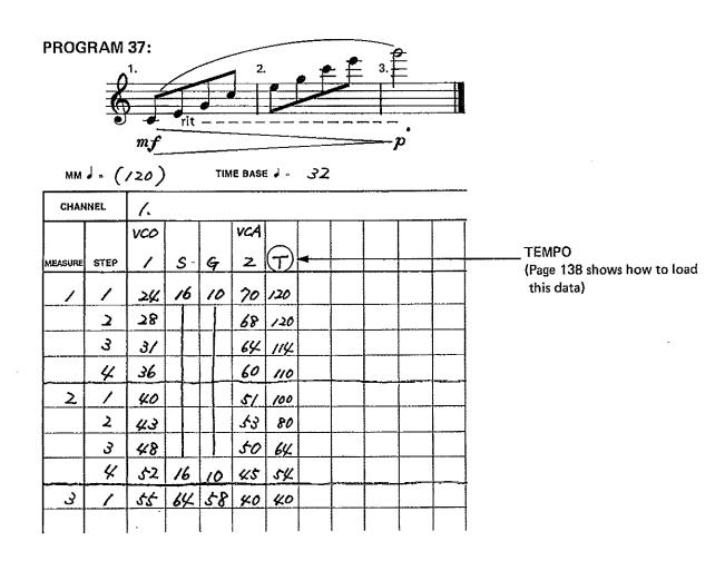
If the full eight channel output is not being used, it may prove better to assign TEMPO to an unused channel rather than combining it with a CV channel. Using a separate channel makes it easier to program sections where tempo changes do not occur and is more economical of memory space; combining TEMPO with a CV channel means that all steps in that channel must also be loaded with a TEMPO value as well as pitch value.
