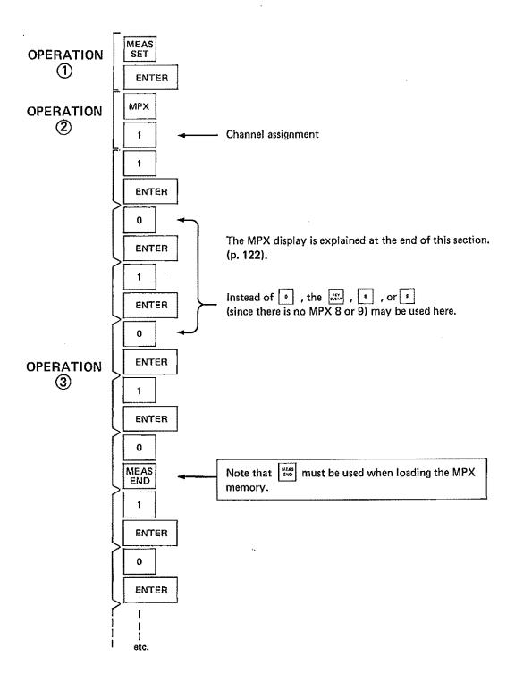
Up to this point the use of the multiplex over the standard gate output would seem to be a disadvantage since the multiplex requires twice as many steps for the same number of notes. By using multiplex, however, six completely independent rhythm voices can be programmed at the same time using only two memories (one channel): MPX and STEP TIME.
