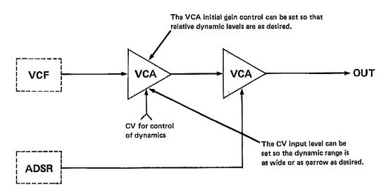
Since VCA controls can be used to control the relative levels and dynamic range, the values loaded into the CV memory are not critical.
