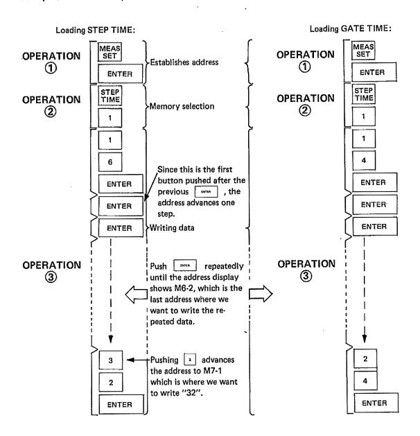
Note that pushing writes into the memory whatever data is displayed by the KEY/MEM DATA display; therefore, can be used for data which repeats.
