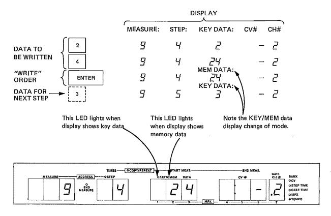
**IMPORTANT:** The first number key pressed in the write operation advances the ADDRESS one step.
