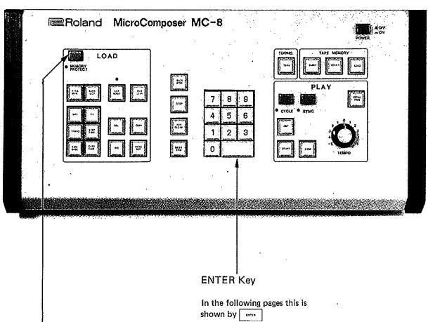
NOTE: None of the front panel controls operate when the MEMORY PROTECT switch is depressed (LED on).
