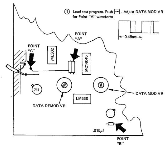
(2) Connect patch cord between TAPE MEMORY DUMP and LOAD jacks. Push . Adjust DATA MOD VR so Points "B" and "C" show the same waveform.
