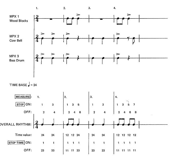
Each rhythm voice is assigned to one of the multiplex outputs; each step in the program is then programmed to contain the multiplex pulses for the rhythm voices which are to sound at that point in the program.
