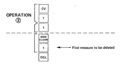
In the above, the assignment of CV1 to Channel 1 remains intact, but CV1 now contains no data. The ADDRESS display will show M0 (measure zero) and the KEY/MEM DATA display will show "0". Remember that the MicroComposer will not run in this condition; data must be reloaded into CV1, or the channel assignment must be cleared.
