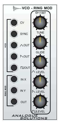
What the RM does is take 2 audio inputs, which we will call X and Y, then produce an output that contains the original frequencies X and Y, as well as the sum and differences of X and Y (X+Y, X-Y).
