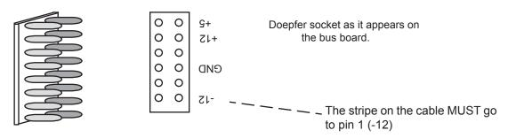
The socker on the lead may have more holes than there are pins on the PCB. On allConcussor modules, there are 12 pins on the board, and either 14 or 16 holes in the socket. The same applies though - match the striped end of the lead/socket to the work 'STRIPE' on the board. In this case the socket will over hang the board on the opposite end to the stripe end.
