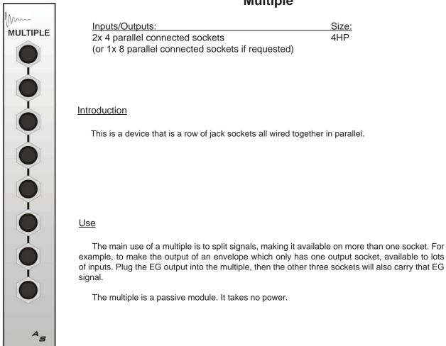
When a signal is split by a passive device such as a multiple, the output power level will be reduced. This generally will not cause a problem as most modules' inputs are buffered.
