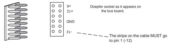
The socker on the lead may have more holes than there are pins on the PCB. On allConcussor modules, there are 12 pins on the board, and either 14 or 16 holes in the socket. The same applies though - match the striped end of the lead/socket to the work 'STRIPE' on the board. In this case the socket will over hang the board on the opposite end to the stripe end.
