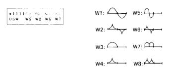
These waveforms can be used as both carriers and modulators. Sine waves (waveform 1) are pure tones. The other seven waveforms have additional harmonics already in them. This allows for complex waveforms to be created from fewer operators. For ideas on how to use the various waveforms, examine the preset voices. The harmonic content of each waveform is described on p.25.
